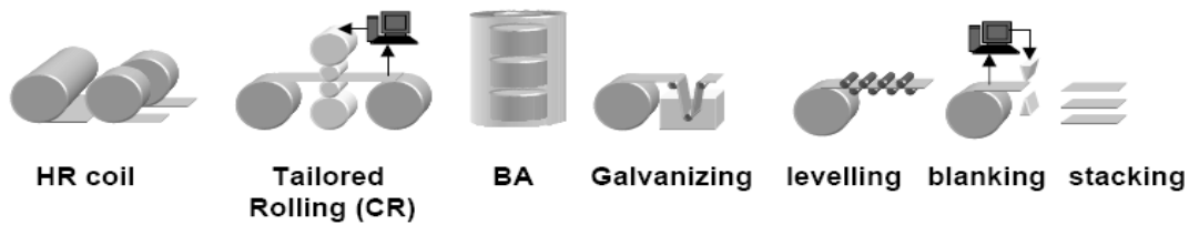
Figure 11 [5, 35] : Tailor Rolled Blanks production process.
