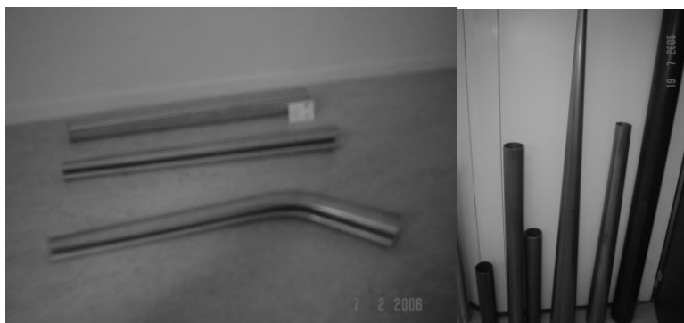
Figure 4 [6, 16] : Tubes made with Tailor Tube Process
